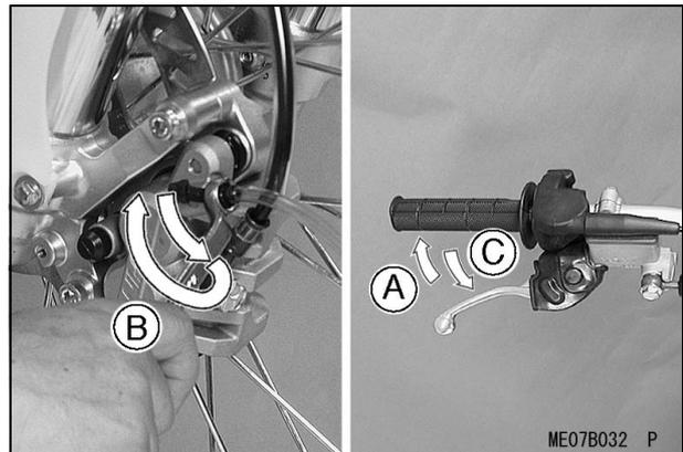
**A. Hold the brake lever applied.**
